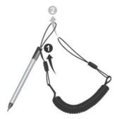
2. Insert the other loop end to the hook on the computer (as indicated by below). Then, insert the stylus end through the loop (as indicated by below) and pull it tight.
