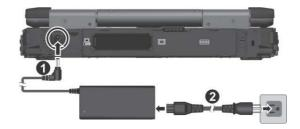
3. Power is being supplied from the electrical outlet to the AC adapter and onto your computer. Now, you are ready to turn on the computer.
