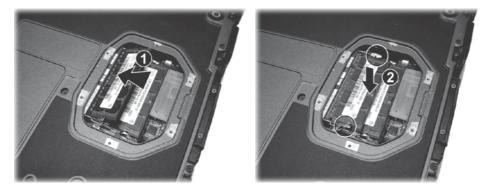
**CAUTION:** If the RAM module is difficult to insert or difficult to push down, do not force it. Check once more to ensure that the module is positioned correctly.
