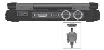
**NOTE:** Portable modems that derive power through the serial port cannot be used with the computer. Instead, use a modem that is powered by its own internal battery or external AC power.
